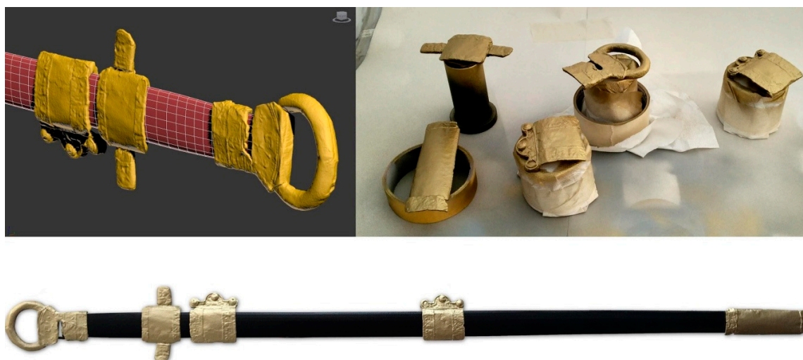
Figure 28. 3D printing of the Kunàgota sword: Mesh optimization; 3D printing of the models and spraying; completed physical replica of the sword.
