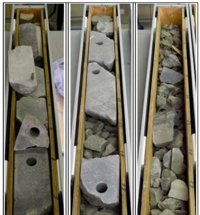
Fig. 8. Some examples of available reservoir well-cores provided by ENI. Cores consist of both blocks and incoherent material, due to the intense state of fracturing in the interval in which the core was taken. In the intact blocks, the circular holes correspond to the core plugs on which porosity and permeability measurements were performed.
