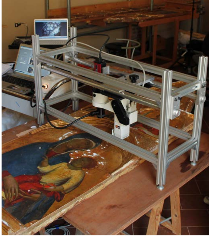
Fig. 1. 3D microscopy inspection of a panel painting by Simone Martini: experimental setup.
