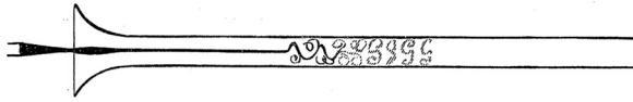
FIG. 5. Reynolds' sketch showing the loss of the laminar regime observed through his experimental apparatus. The thin ink line transported by the fluid rightward abruptly changes, forming more or less distinct curls. 36
