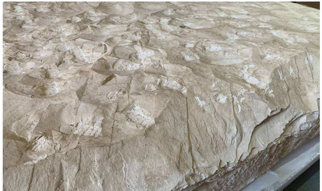
Figure 4. Closed, subparallel microfracture systems, with centimetric spacing, visible on the reverse of the stele.
