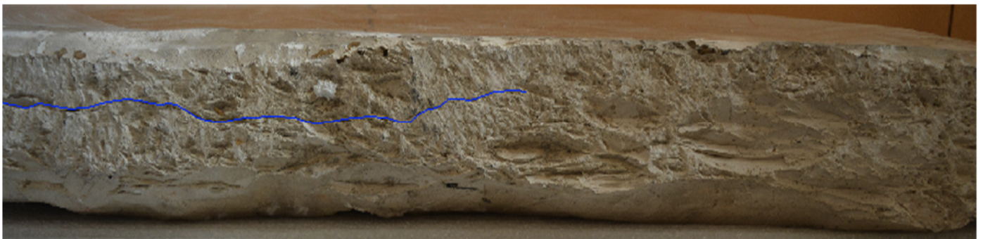
Figure 7. Lateral picture of the stele, showing (in blue) the direction of the crack, which is subparallel to the sedimentation.
