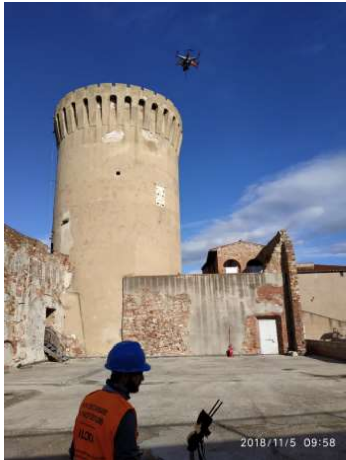
Fig. 2 – The operator pilots the UAV around Mastio di Matilde, a tower in the Fortezza Vecchia complex in Leghorn, which has been considered as a case study in the framework of the Moscardo project.
