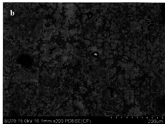
Figure 4: SEM micrograph for samples a) %2,5Cu-%7,5Fe (NTC 2), b) %7,5Cu-%2,5Fe (NTC-4)
