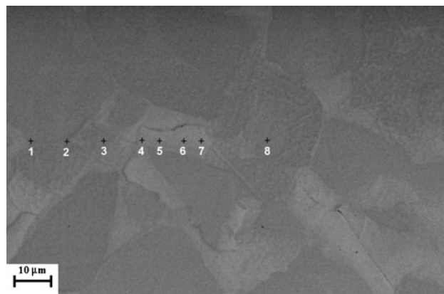
Fig. 2. BSE SEM image of an area of the ISC sample where the compositional analysis, reported in Table I, was performed.
