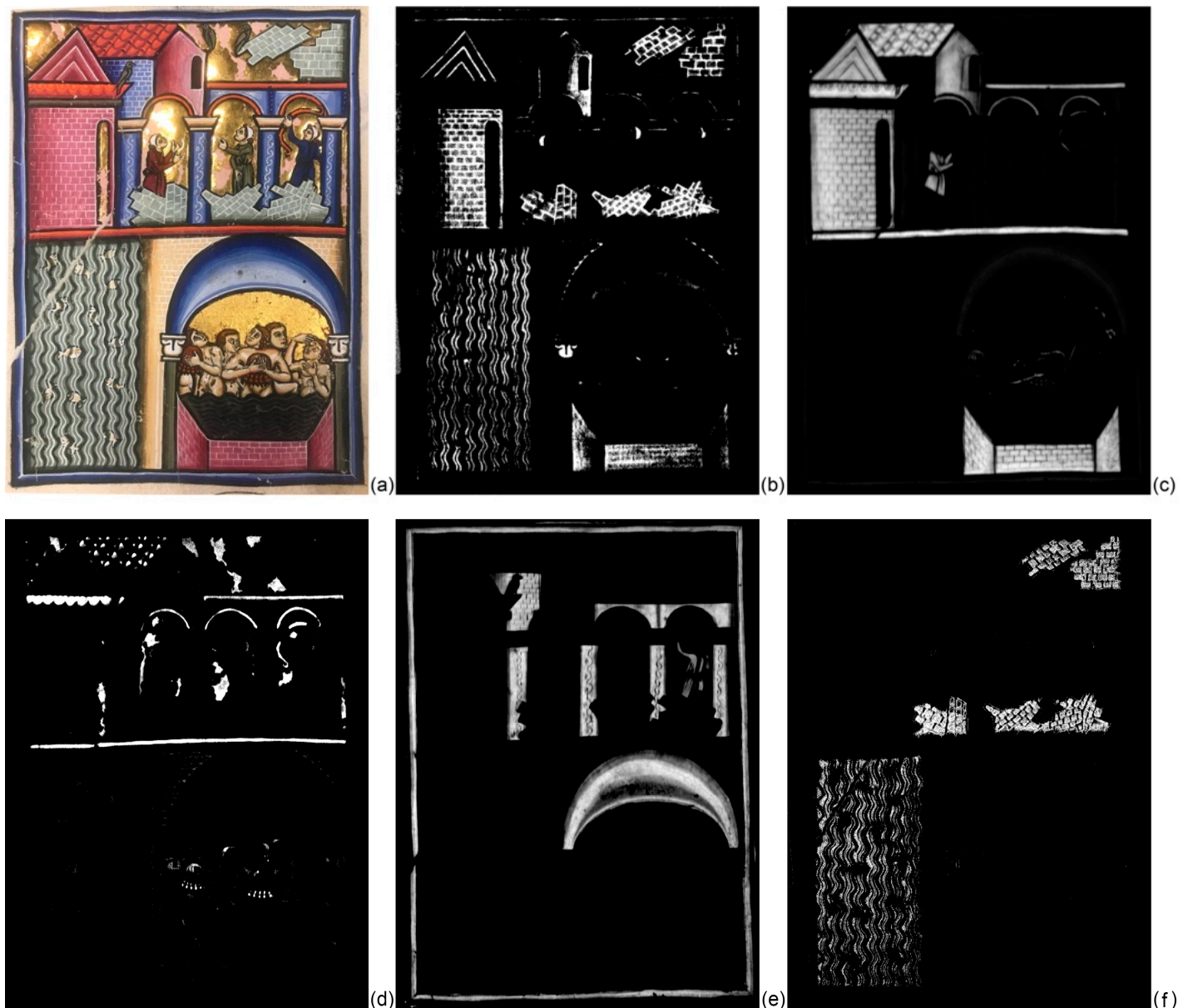
Figure 11. Picture of the illumination (a) and hyperspectral maps of lead white (b), red lake (c), vermilion (d), ultramarine blue (e), and copper-based pigment (f).
