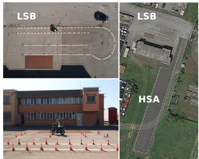
Fig. 1. The motorcycle driving licence test takes place on predefined paths delimited with traffic cones: one path is smaller with close passages and low speed (Low Speed Balance - LSB) and the other is larger and requires higher speeds (High Speed Agility - HSA). On both of them, there is a slalom at the beginning, then a curve, and finally, a straight section. The driver must stop the vehicle in a specific space on the long track. Everything must terminate respecting time constraints. The picture shows the two tracks at the testbed site, the AUG of Pontedera.
