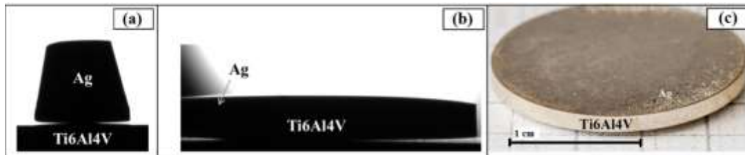
Fig.12- Ag/Ti6Al4V profiles of the sample step-heated: at 850 °C (a) and at 970 °C (b); image of a sample after the wetting test at 1050 °C (c).
