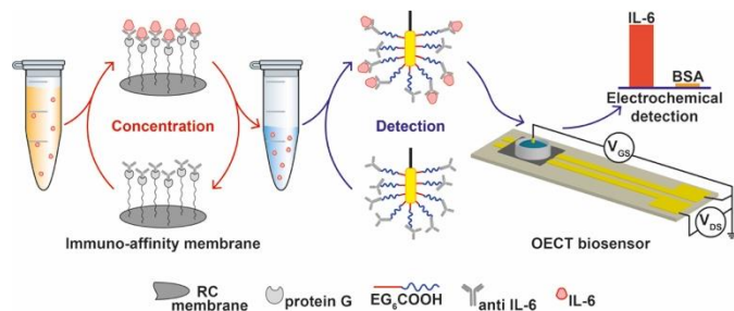
Fig. 1. Schematic illustration of the selective concentration and electrochemical detection of IL-6
