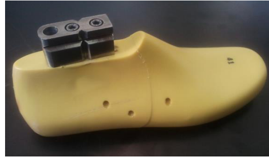
Fig. 2. Last coupled with gripping device
