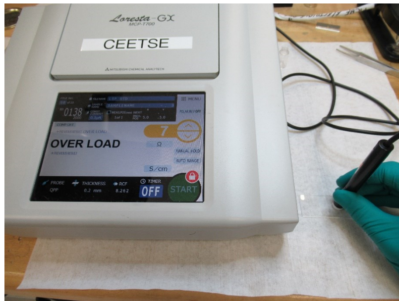
Fig. S2 Four-point probe test of pLAMPnf. The value is out of the range of the instrument ( >10^8 \Omega/\text{sq} ).
