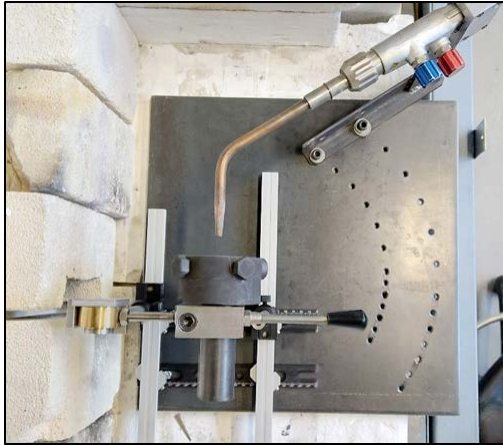
Figure 1: Plan image of variable angle torch test rig. The angle and sample x-y co-ordinate centre may be varied using the array of drilled holes to ensure precise angle and test distances.
