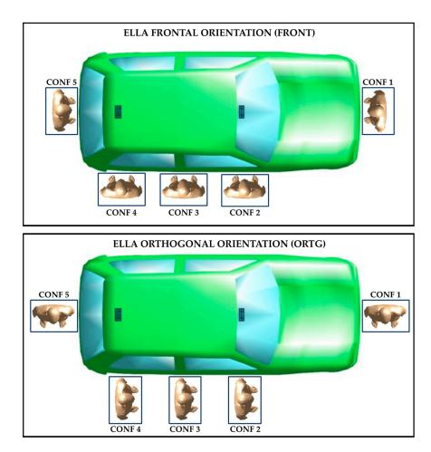
**Figure 2.** The exposure scenario with the car model, the phantom Ella at the five analyzed configurations and the two antenna arrays (the small dark rectangles at the front and rear of the car). The Ella model is placed in the 'FRONT' (**top** panel) and 'ORTG' orientation (**bottom** panel) with respect to the car body.
