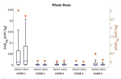
**Figure 6.** SAR<sub>10g</sub> (left *y*-axis, box plot) and  $pSAR_{10g}$  (right *y*-axis, square symbols) in the brain tissue for the five different examined configurations, considering the frontal and orthogonal orientations of the Ella model. The center line in the boxes is the median; the bottom and top edges are the 25th and 75th percentiles. The lower whisker extends to the minimum value, while the upper whisker extends to 1.5 times the height of the box.
