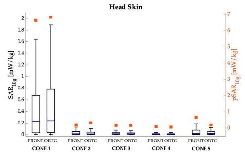
**Figure 5.**  $SAR_{10g}$  (left *y*-axis, box plot) and  $pSAR_{10g}$  (right *y*-axis, square symbols) in the skin tissue over the whole body for the five different examined configurations, considering the frontal and orthogonal orientations of the Ella model. The center line in the boxes is the median; the bottom and top edges are the 25th and 75th percentiles. The lower whisker extends to the minimum value, while the upper whisker extends to 1.5 times the height of the box.
