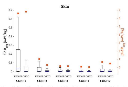
**Figure 4.**  $SAR_{10g}$  (left *y*-axis, box plot) and  $pSAR_{10g}$  (right *y*-axis, square symbols) in the skin tissue over the whole body for the five different examined configurations, considering the frontal and orthogonal orientations of the Ella model. The center line in the boxes is the median; the bottom and top edges are the 25th and 75th percentiles. The lower whisker extends to the minimum value, while the upper whisker extends to 1.5 times the height of the box.
