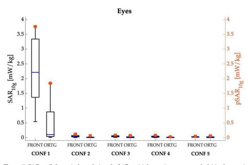
**Figure 7.**  $SAR_{10g}$  (left *y*-axis, box plot) and  $pSAR_{10g}$  (right *y*-axis, square symbols) in the eye tissues for the five different examined configurations, considering the frontal and orthogonal orientations of the Ella model. The center line in the boxes is the median; the bottom and top edges are the 25th and 75th percentiles. The lower whisker extends to the minimum value, while the upper whisker extends to 1.5 times the height of the box.
