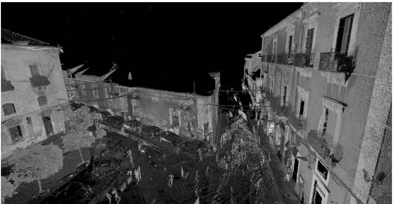
Fig. 24 Perspective view of the point cloud of the minor building in Catania's historic centre.
