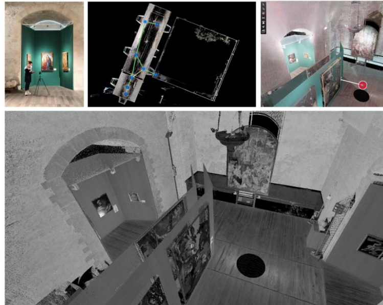
Fig. 15 Pinacoteca of the Civic Museum Castello: panoramic image survey performed with BLK360.
