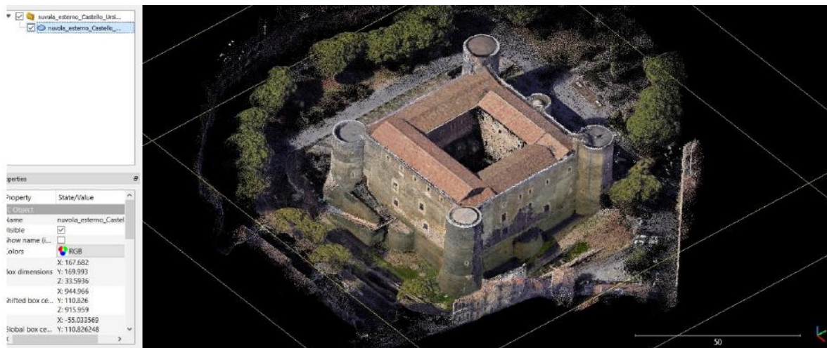
Fig. 16 Point cloud perspective view obtained from a photogrammetric survey of the exterior of the Museo Civico Castello Ursino in Catania.
