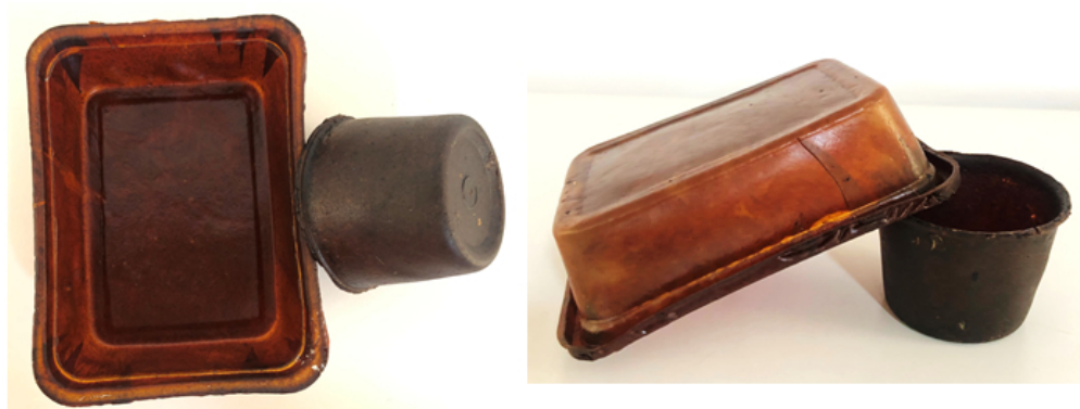
Figure 9: Three-dimensional cups and boxes suitable for food and non-food packaging have been developed from pongamia protein, demonstrating the feasibility of preparing bioproducts for commercial applications.
