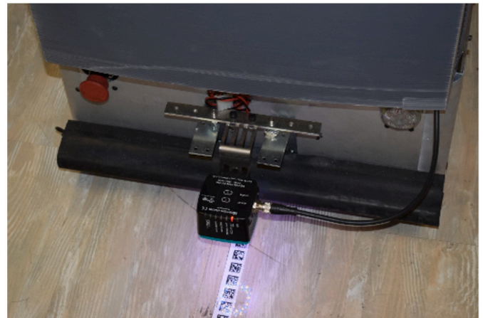
Fig. 13. The PGV read-head in the process of following the routing tape.
