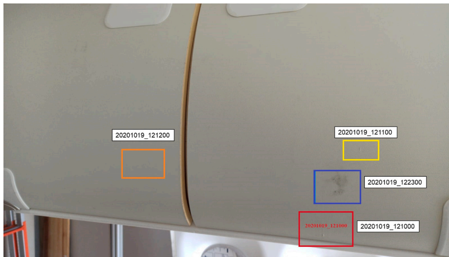
Fig. 17. Surface anomalies can be detected with both 3D and color cameras, with each one providing benefits in specific cases. For instance, subtle surface issues like the scratch in the orange box are better handled by the 3D acquisition and processing pipeline.
