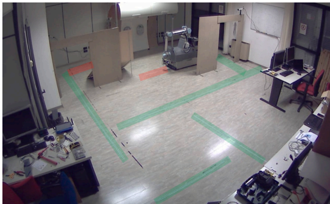
Fig. 11. VISTA partners facilities testing room. Position of the routing tape is highlighted in green and red. Green lanes are transit area on which the testing system moves to reach the inspection areas, where the lanes are instead highlighted in red. The AGV follows the lanes using the PGV optical head once properly programmed.
