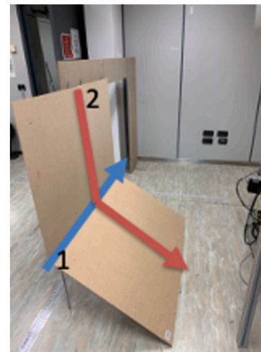
Fig. 12. Example of an inspection plan related to the cargo area, composed of two basic single profile working plans.
