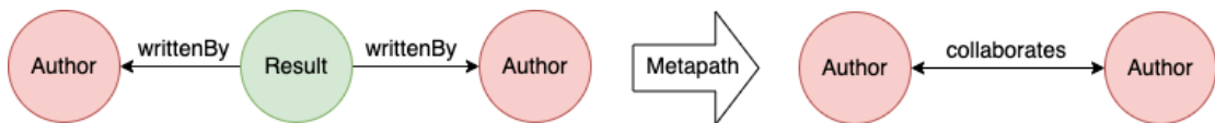
Figure 5.7: Metapath example: the heterogeneous graph with publications and authors has been transformed into a homogeneous graph with only author node types.
