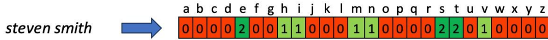
Figure 5.2: Simplified example of the encoding computed with the “bag of letters” model (in this case the dictionary includes only letters of the alphabet for better visualization).
