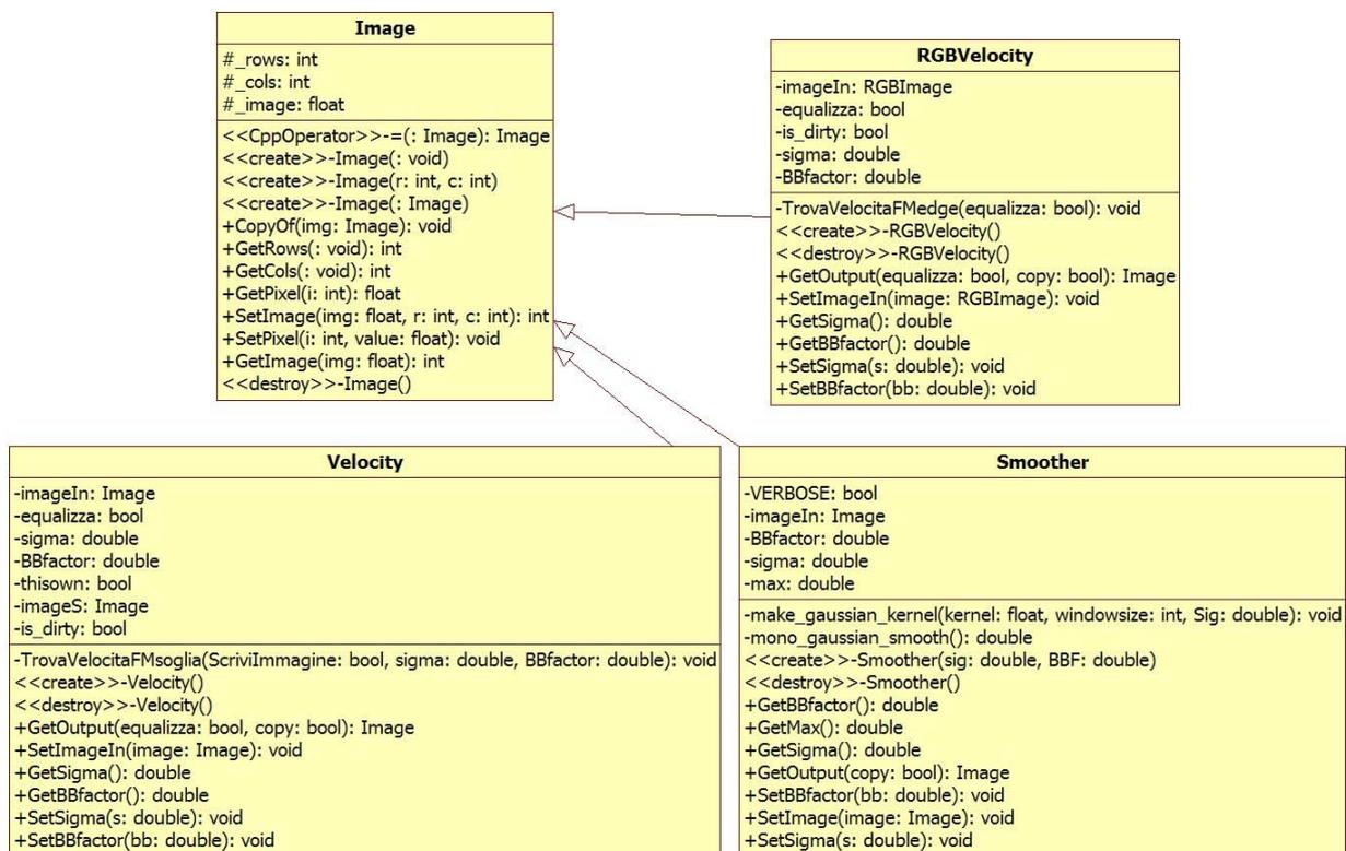
Figura 3-3: RGBVelocity, Velocity, Smoother derivate da Image
