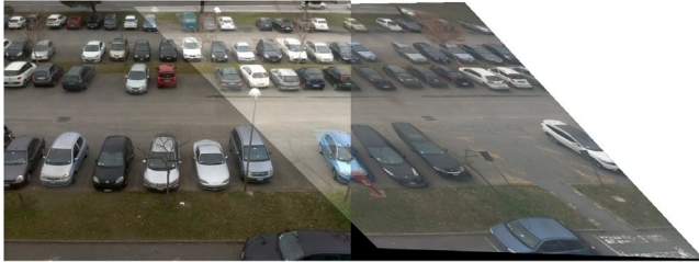
Fig. 3. Example of concatenation of two images using a homographic transformation, where it is also visible the overlapping area between them.
