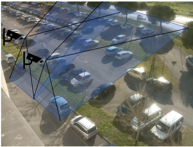
Fig. 1. An example of two cameras monitoring the same parking area with partially overlapping fields of view. This redundancy provides robustness and fault-tolerance but also raises the problem of aggregating knowledge extracted from the individual cameras.
