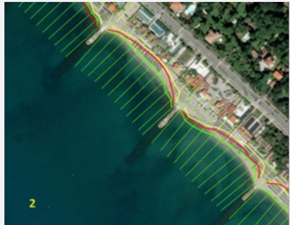
Figure 27: Results of coastal shoreline erosion projections for Massa beach
