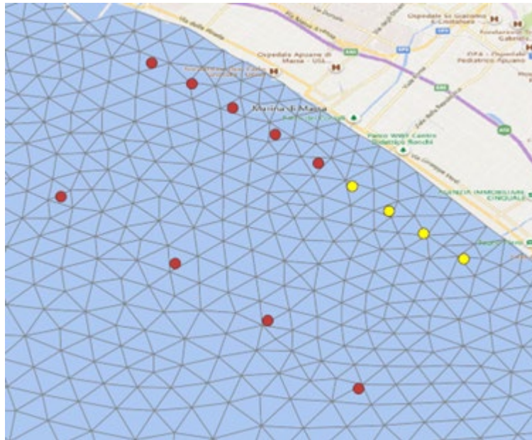
Figure 26: Detail of WW3 unstructured grid used for wave downscaling. Wave climate data were extracted from the yellow nodes.
