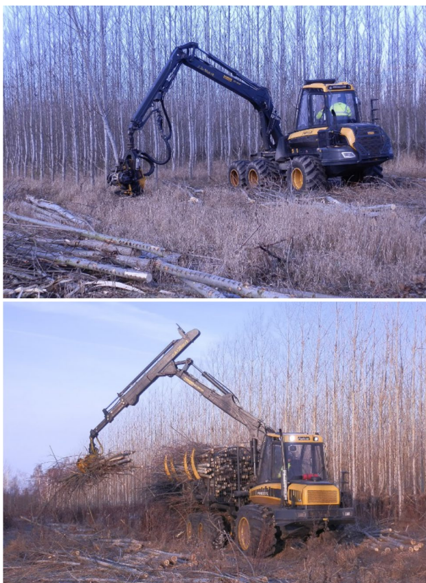
Fig. 1 Two machines tested in Gardeja: harvester (top); forwarder (bottom)
