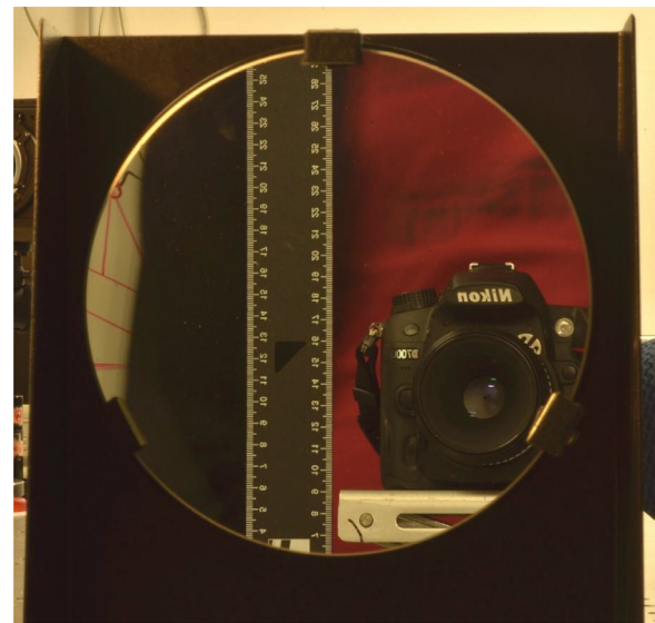
Fig. 4. Photo of a ruler taken through the concave mirror.
