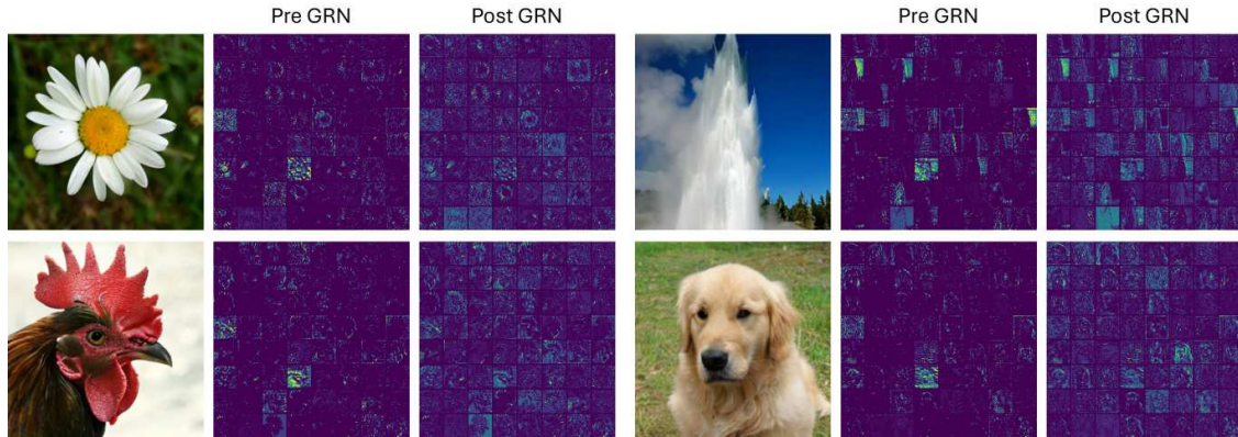
Figure 7. Feature activation visualization. We visualize features before and after the GRN layer during sampling for each image on the left. The first 64 channels of the last block in the first stage are shown as 8×8 grids. GRN clearly reduces channel redundancy.
