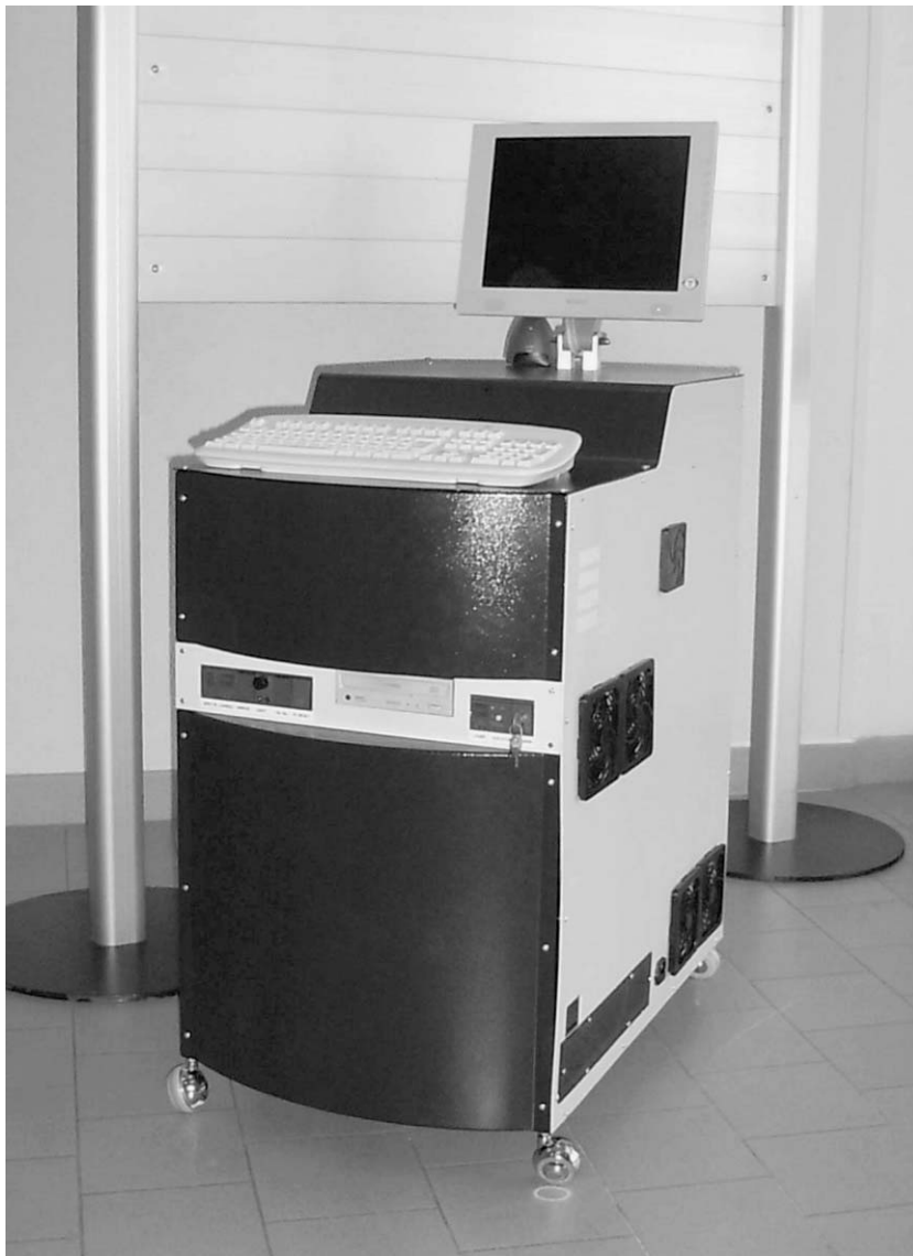
Fig. 1. The mobile dual-pulse instrument (MODI) for LIBS environmental applications developed at the Applied Laser Spectroscopy Laboratory of IPCF in Pisa.
