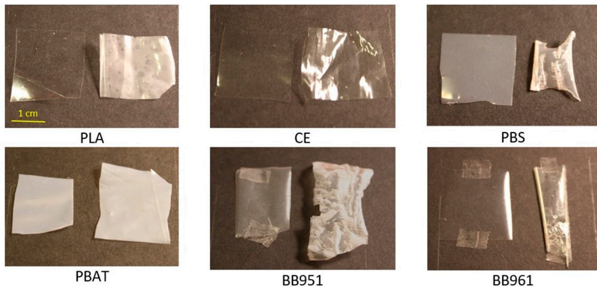
Figure 1. Pictures of the bioplastics before ( left ) and after ( right ) exposure to MilliQ water for 3 h at 80 °C. The treatment modifies the transparency properties of the polymers, sometimes in a severe way. In the best cases (CE and PBAT), only some wrinkling is observable. For bilayer materials, a mismatch in the shrinking of the polymer sheets is also observed.
