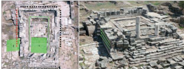
Fig. 2. Building A, left: acquisition geometry for seismic refraction tomography (geophones = red points; shots = black points) and GPR profile location (1 = area of profiles R7-R18; 2 = area of profiles R19-R30); right: GPR profile location on the northern side of the podium.
