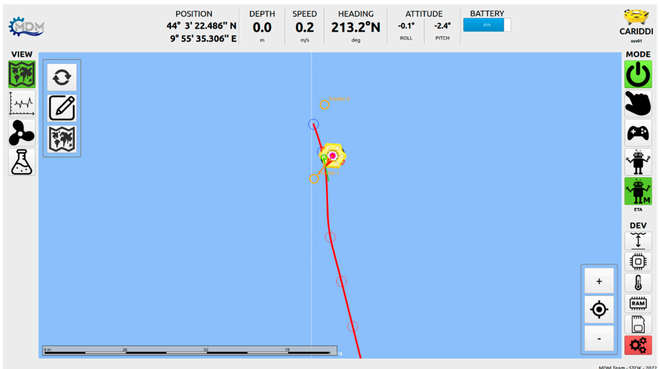
Figure 5. The primary drifter is following the central position of two secondary drifters (orange circles), following a trajectory (red line) computed interpolating predictions of the centroids (circles on the trajectory).
