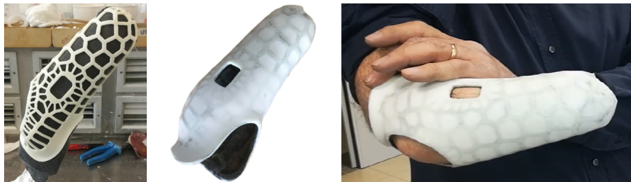
Fig. 3. Left: Hypermat metastructure just before the lamination process. The black knit sleeve of Nylon/Perlon modified with rGO is visible. Middle: Hypermat metastructure embedded in the resin modified with PCM after the lamination process. Right: Volunteer wearing the prototype of the prosthesis socket. The socket weighed 165g.
