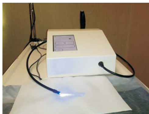
Figure 1 Photo-hemostatic device. The picture shows the optimized first LED fiber coupled photo-hemostatic device, with software control of emission power and treatment time duration.
