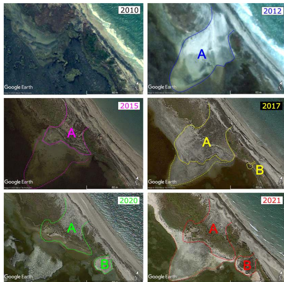
Figure A8. Formation and accretion of the washover fans A and B (cf. Figure 10). The dotted lines mark the submerged edge during high tide conditions. Note the black sediments that mark the shape of the backshore and the sea and lagoon shorelines ( 40^{\circ}21'25.14'' – 40^{\circ}21'29.31'' N, 18^{\circ}20'26.17'' – 18^{\circ}20'33.10'' E; eye elevation of 128 m).
