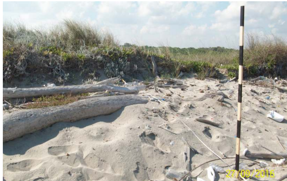
Figure 11. Measurements of dune width and height ( 40^{\circ}22'06.85'' N, 18^{\circ}19'30.30'' E) 27 September 2016; graduated rod, placed at the dune toe, is subdivided in 20 cm-long segments. The height of the dune ranges here from 0.9 to 1.1 m, the maximum value found in the northwest sector. The distance between dune toe and vegetation line is 2 m.
