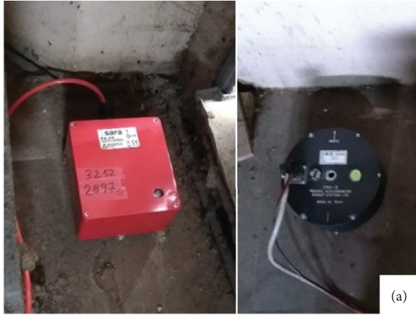
FIGURE 6: (a) A velocimeter and an accelerometer installed on the bell tower; (b) velocities recorded by using the SS20 2045 seismometer during Experiment 0.
