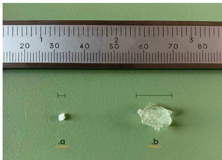
Figure 1. Dry (a) and hydrated (b) potassium polyacrylate hydrogel.
