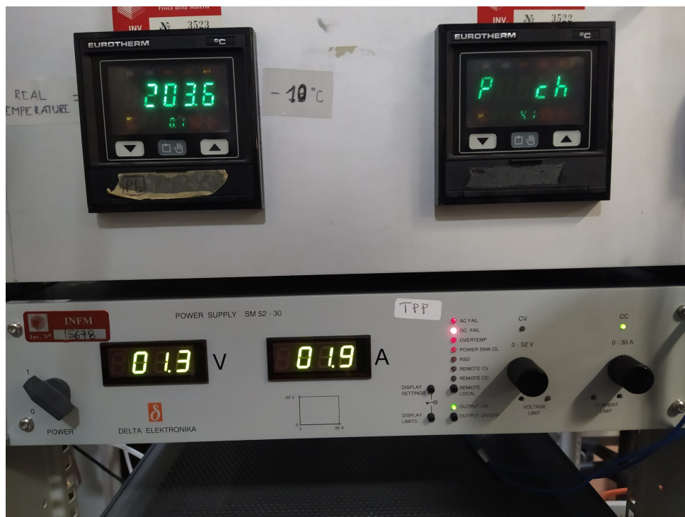
Figure 38: MBE power supply and temperature reading.
