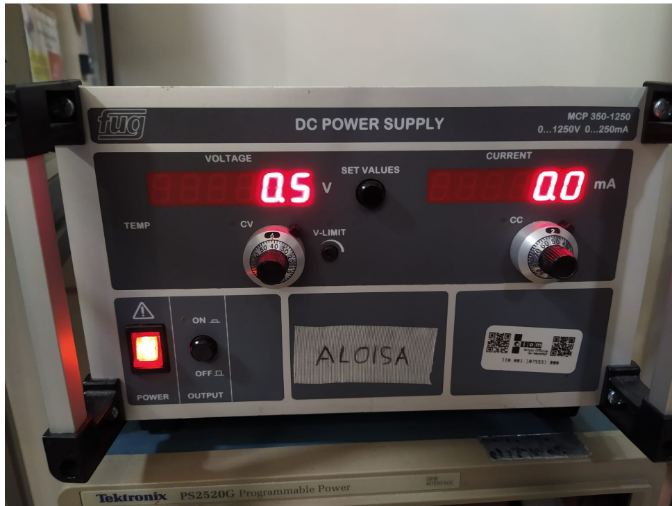
Figure 35: High Voltage power supply.
