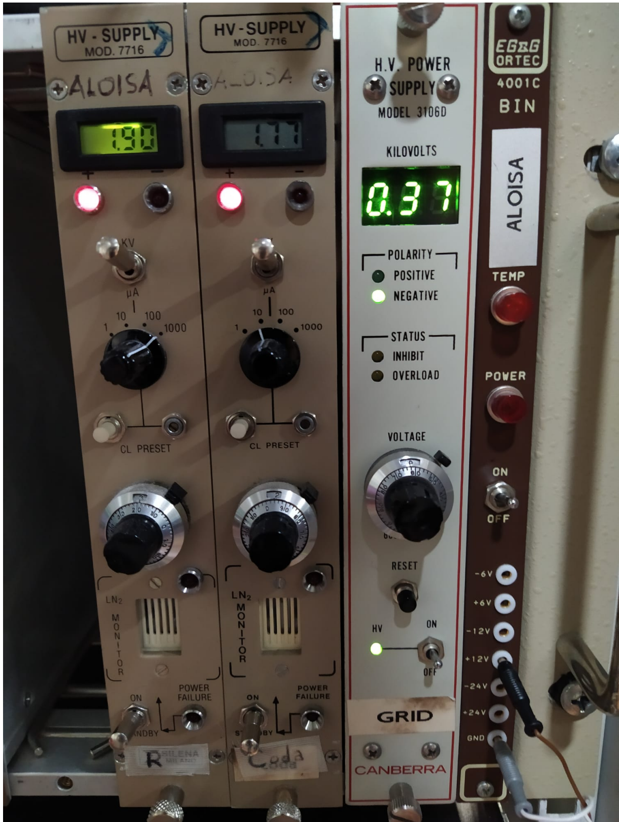
Figure 23: The channeltron multiplier power supplies. From left to right: Channeltron electrode, channeltron back, channeltron grid.
