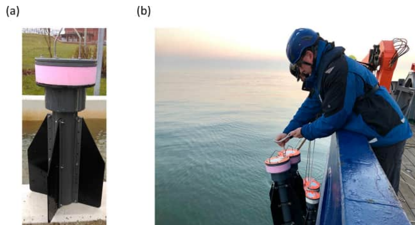
Figure 4.9.3. One of the GPS drifters (a) and their deployment (b) during the RV Heincke cruise HE503 at Borkum Riffgrund (Meyerjürgens et al. 2019).
