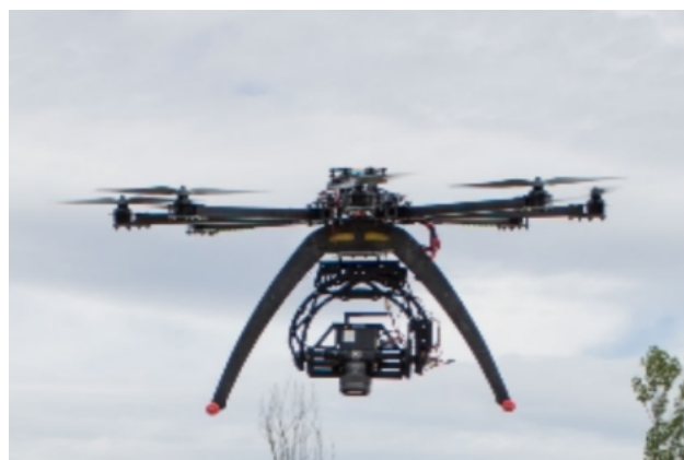
Figure 3. The ISTI-CNR drone: the digital camera is hosted by the gimbal, a mechanical support able to stabilize the image acquisition against vibrations or unexpected movements.
