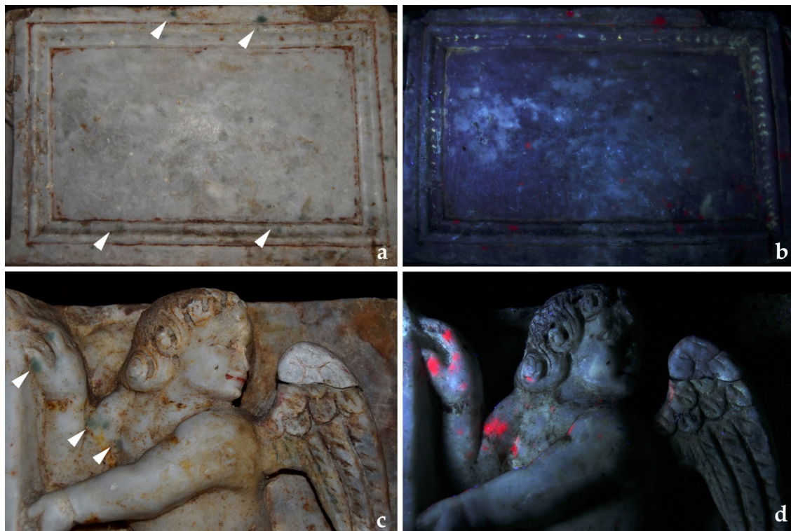
Figure 2. (a) Vis and (b) UVL images of the tabula and (c) Vis and (d) UVL images of cupid2. First register of the sarcophagus. The arrowheads indicate the blue–green biological growth.
