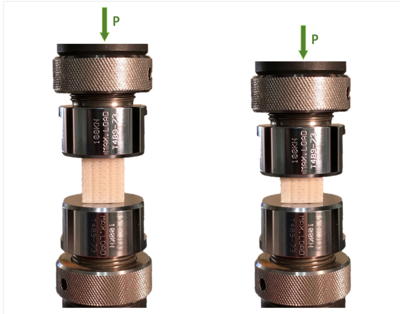
Figure 4: Compression tests on 3D-printed cellular structures.
