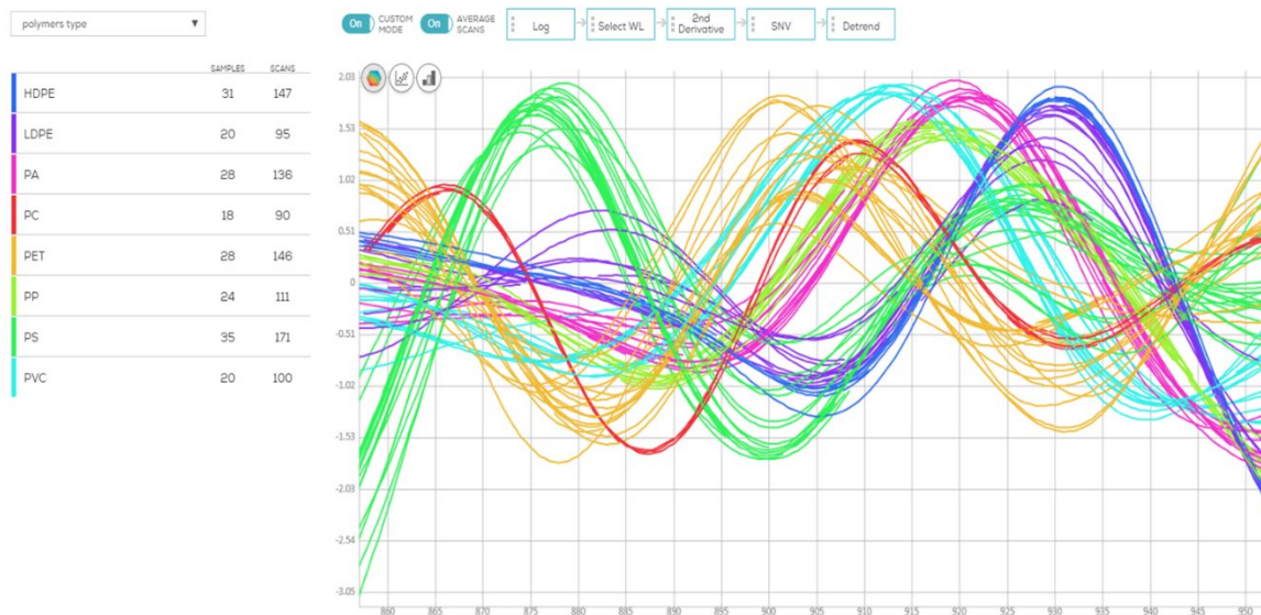
Figure 17 Spectra from the polymers after data treatment (log, average, 2 nd derivative) from the selected wavelength range of 850-950 nm.
