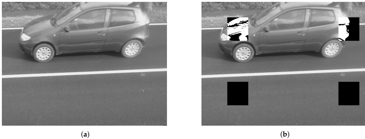
Figure 8. Traffic flow analysis: detected vehicle from sensor test set-up (a) and the same frame processed with the RoIs highlighted (b).
