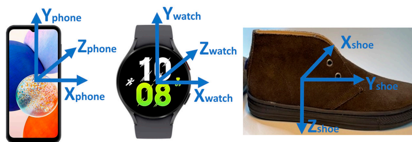
Figure 1. Smartphone (left), smartwatch (center), and smart shoe (right). Local reference frames associated with the inertial sensors are reported.
