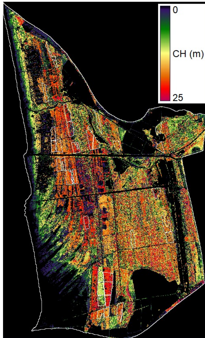
Figure 5. ALS CHM of May 2015 with with superimposed boundaries of the park area and of the 32 selected forest stands (while lines).
