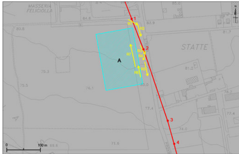
Figure 6. General map of the investigated area, showing in red the route of the Triglio aqueduct and the location of the shafts 1–4, in yellow the GPR profiles R1–R7, and in light blue the area surveyed using electrical resistivity tomography (ERT) (A).
