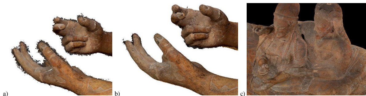
Figure 8. a) Noisy points generated from mixed pixels on boundaries. b) The erroneous points are reduced when all the images are used together. c) Particular of the photogrammetric textured 3D model.
