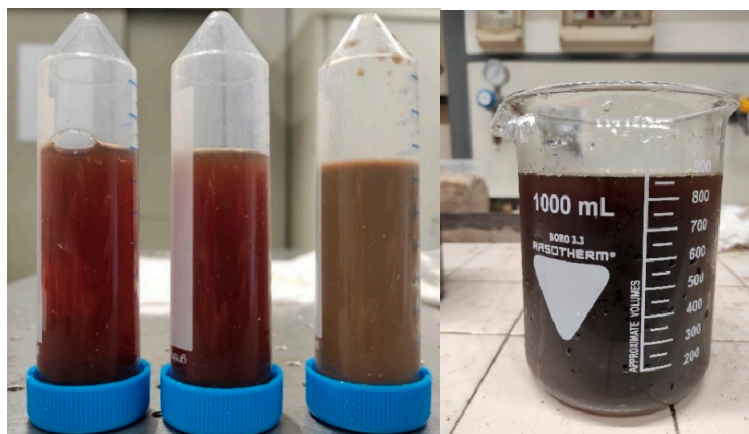
Figure 5. The left picture shows samples S120, S500 and US collected for COD measurement; in the right picture is the vegetation water filtered and neutralized at pH 5.5.
