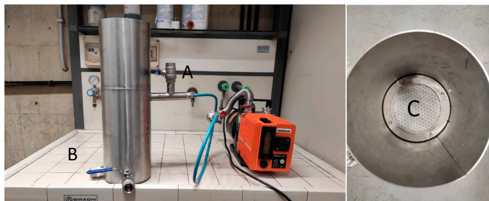
Figure 1. Experimental filter for the removal of suspended solids from vegetation water: (A) hydraulic valve connecting the lower chamber with a vacuum pump; (B) filtered water drain valve; (C) top vision of the filter with the supporting technical sheet.
