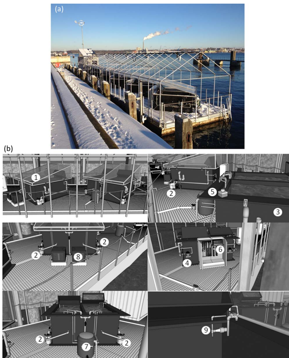
Fig. 2. (a) Overview of the Kiel Outdoor Benthocosm infrastructure showing the six tanks with their subunits covered by hoods as well as (in the background) the technical container bearing on its roof the solar panels and the wind generator. (b) Sketches of important functional components of KOB. Not shown are the numerous IT components. 1: hood, 2: circulatory pumps, 3: position of lateral ports, 4: measurement cell, 5: p\text{CO}_2 sensor, 6: measurement and control unit, 7: heat exchanger, 8: coolers, 9: water inflow (and air injection (not shown)).
