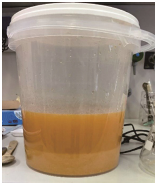
Fig. 1. The aqueous mixture of red orange citrus processing waste (CPW) used for CytroCell and IntegroPectin extraction via acoustic cavitation.
