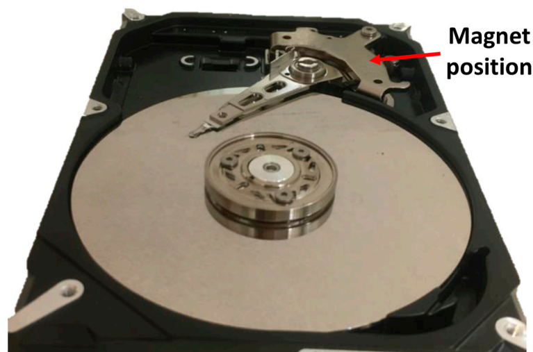
Figure 1. Hard disk drive with the magnet position.
